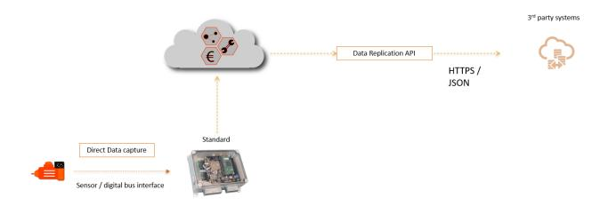
The high-level idea is to trigger data transfer to the customer's own data storage system at the same rate metrics are received into the Condence cloud system from the smart terminals in the field. This process is called here as data replication.
